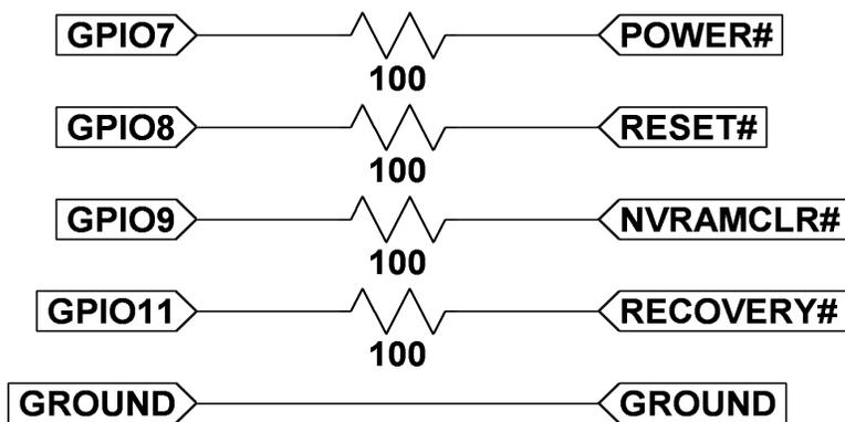
Recommended external SPI firmware connection method for targets with DIP-8 / SIP-8 Flash devices:
