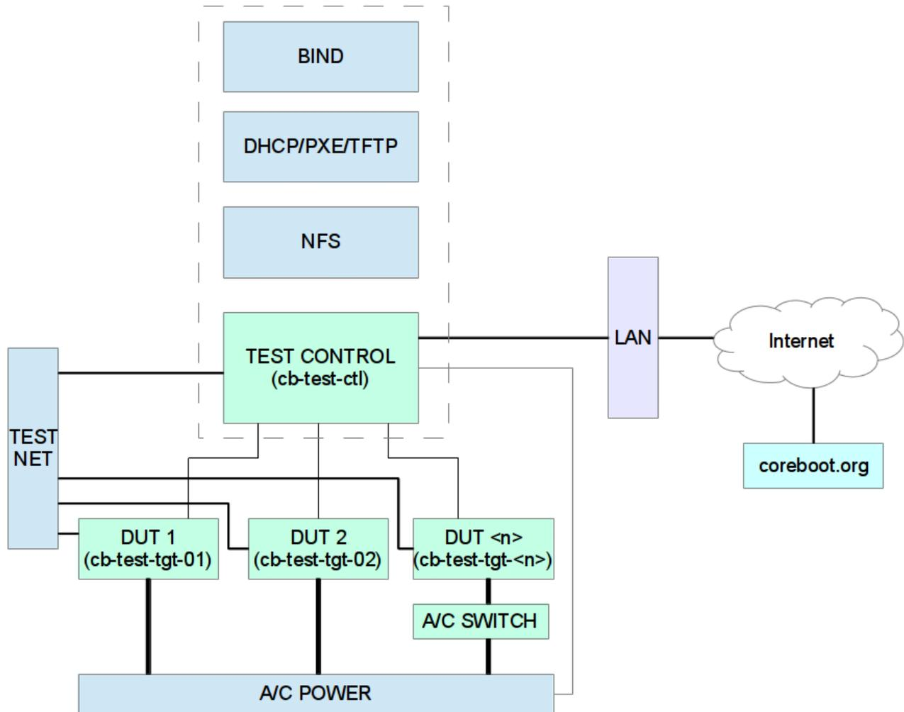
Fig. 1.1 Simplified Diagram of Automated Test Stand
